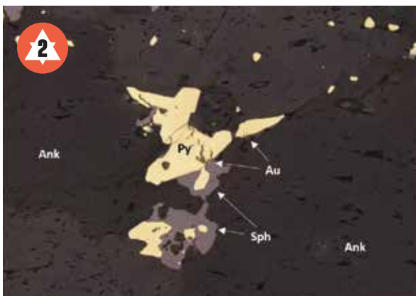
Fig. 2: Refl_photomicrograph: Photomicrograph image of gold-bearing rock showing multiple metallic minerals in a carbonate matrix with trace gold mineralization. 40x magnification. Plane-polarized reflected light. Ank = ankerite. Py = pyrite. Sph = sphalerite. Au = gold.
